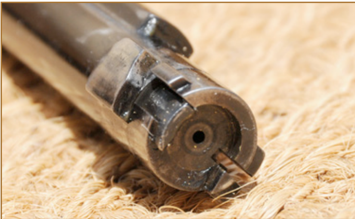
Detail on the occluded firing pin section on the bolt
