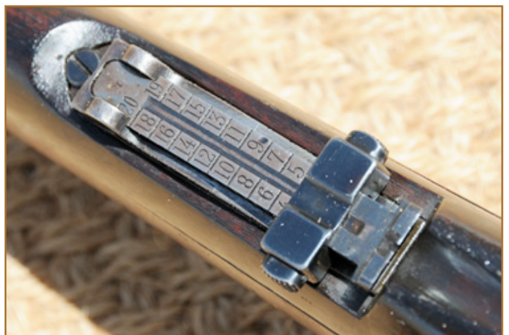
Perspective on the 20 position marked scale for the elevation adjustable sight
