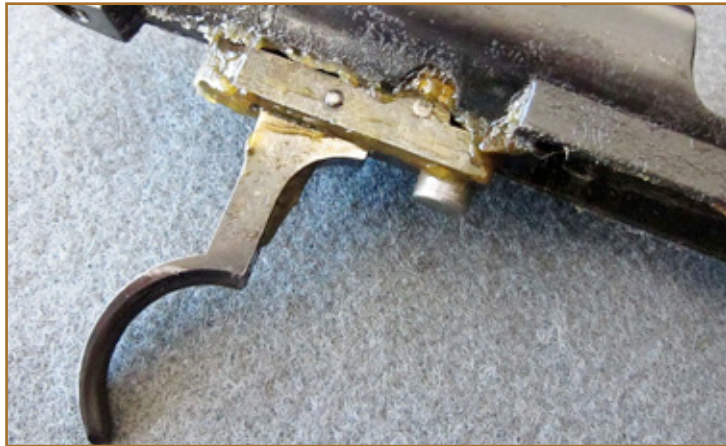
Detail on the trigger block after field stripping the action and barrel from the stock – the generous amount of conservation paste demonstrate the original state as this Vergueiro was received (oriented towards long time storage conservation)
